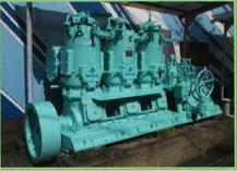
This hot-bulb engine was built in March 1961 by Makita Ironworks (now Makita Corporation). The three-cylinder, 100-horsepower engine was installed in a freight ship used for shipping crushed stone.
